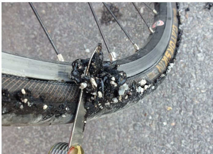
Accumulated melted asphalt and gravel. (photo courtesy Dr. Larry Preble)
