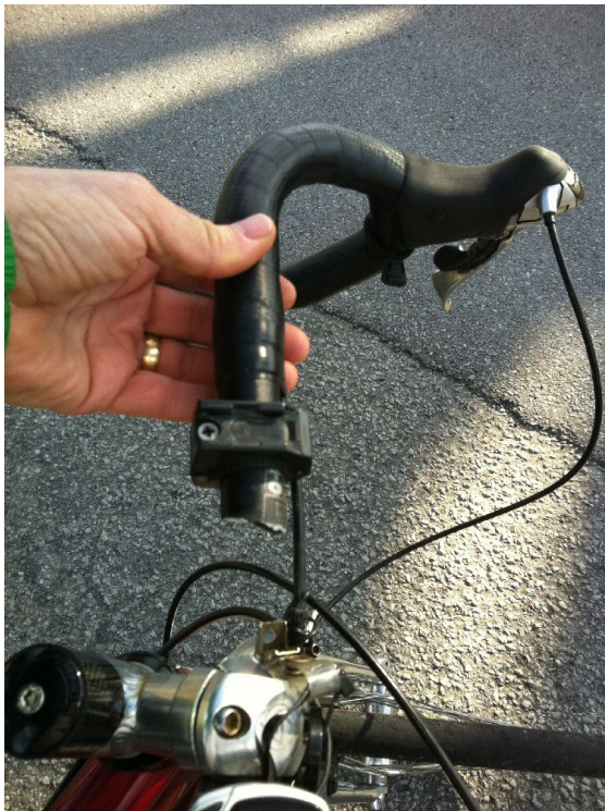
Broken bar (photo courtesy Larry Preble)
