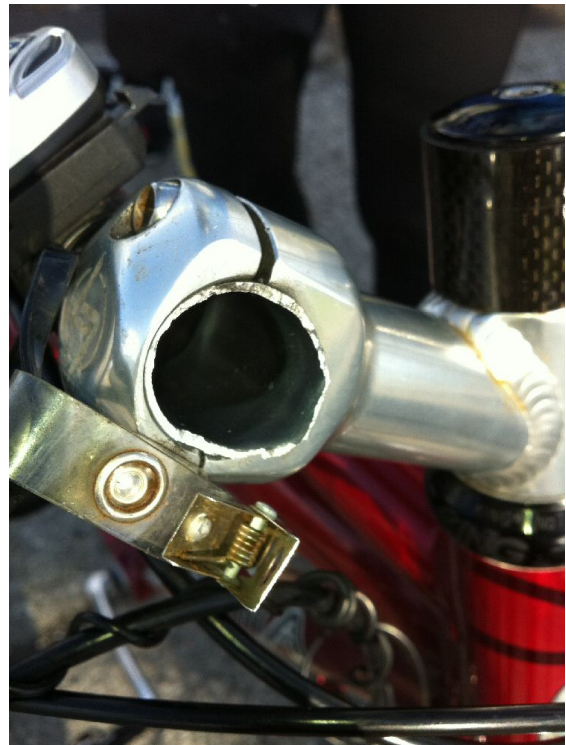
Stem with broken bar (photo courtesy Larry Preble)
